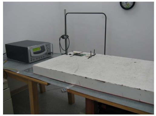
Test Mode : Mode 2: Standby Description : Voltage Dips and Interruption Test Setup
