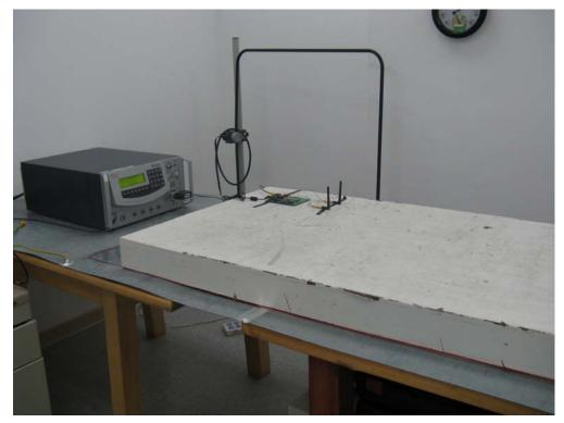
Test Mode: Mode 2: Standby Description: Surges Test Setup for Main
