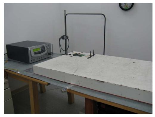
Test Mode: Mode 2: Standby Description: Fast Transients Common Mode Test Setup for LAN
