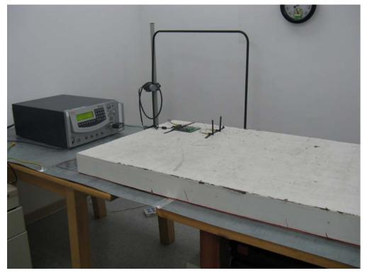
Test Mode: Mode 1: Communication by WLAN Description: Fast Transients Common Mode Test Setup for LAN
