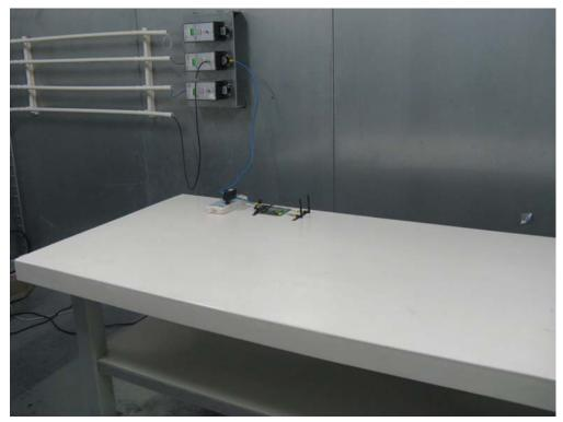
Test Mode: Mode 1: Communication by WLAN Description: Back View of Conducted Emission Test Setup for LAN
