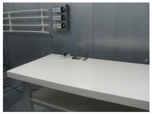
Test Mode: Mode 1: Communication by WLAN Description: Back View of Conducted Emission Test Setup (AC input/output Ports)
